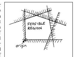
Figure 2.5: The origin is always a feasible cornerpoint in a standard form LP.
