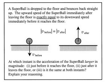
Fig. 1. The *SuperBall problem*. This problem was used on a pretest given in intermediate mechanics after lecture instruction on air resistance.
