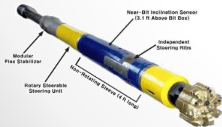
Fig. 5. Rotary Closed-Loop System (RCLS) Bottom-Hole Assembly (Baker Hughes)
