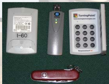
Figure 2. Personal Response System keypads and radio frequency receiver (dark grey). Each keypad was given a unique ID# such as “I-60”.
